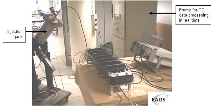
Fig. 1 View of global measurement system of the in-plane permeability bench.
